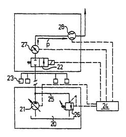
(57) Abstract: Disclosed is a device which is used to supply liquid media to the consumers of a fuel cell system, comprising a feed pump which is considerably more economical in comparison with prior art. Controllable dosing valves (22) are thus provided in between the feed pump (21) and the respective consumers.
